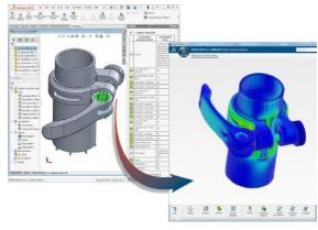
Transfer geometry and model features from SOLIDWORKS Simulation to Structural Professional Engineer with a single click to perform advanced simulation studies.
